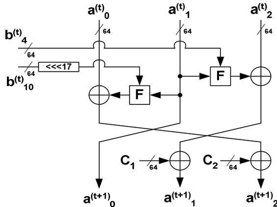
Fig. 4. The  $\rho$  function VLSI implementation
