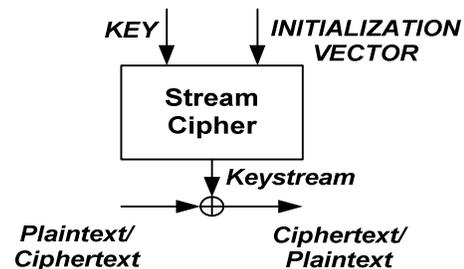
Fig. 1. The stream cipher process
