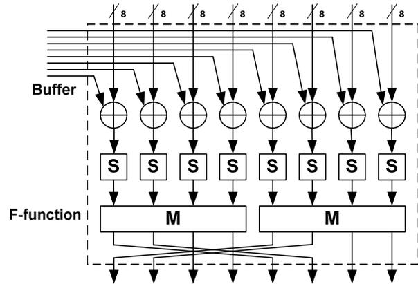
Fig. 5. The F-function hardware architecture
